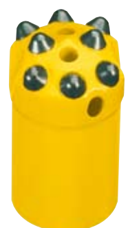
Model -34 All-round bit for soft to hard rock formations. Two front flushing holes for optimal speed and less hole deviation. Front buttons inclined 15°.
