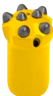
Model -27 All-round drill bit for medium-hard to hard rock formations. Front and side flushing. Diameters from 35 mm.
